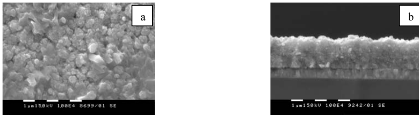
Figure 3. SEM image of the surface (a) and cross section (b) of the ZnO nanostructured film deposited in the conditions with lower \text{H}_2\text{O}_2 concentration with flowing air (sample B).
