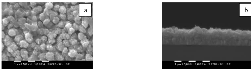
Figure 4. SEM image of the surface (a) and the cross section (b) of the ZnO nanostructured film deposited in the conditions with lower \text{H}_2\text{O}_2 concentration without flowing air (sample C).
