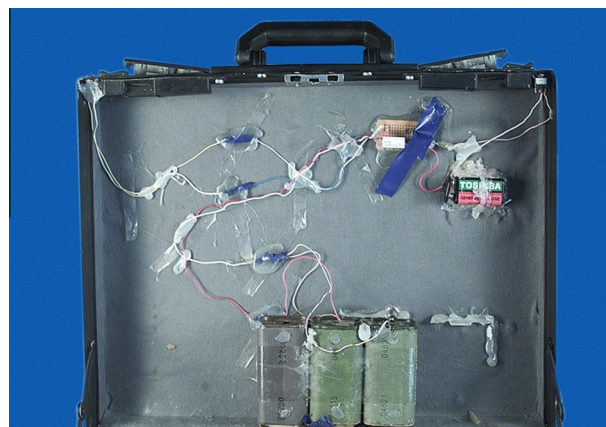
Photo 1 The inner view of on simulated IED inside a suitcase.
