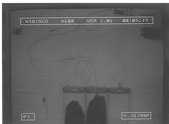
X-ray image 6 The X-ray image with 90°, 99 p and 150 cm distance.
