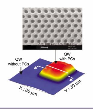
SEM image and near-field scanning optical microscopy (NSOM) intensity image collected above the patterned photonic crystal (PC) region -20 times enhancement under optical pumping.
