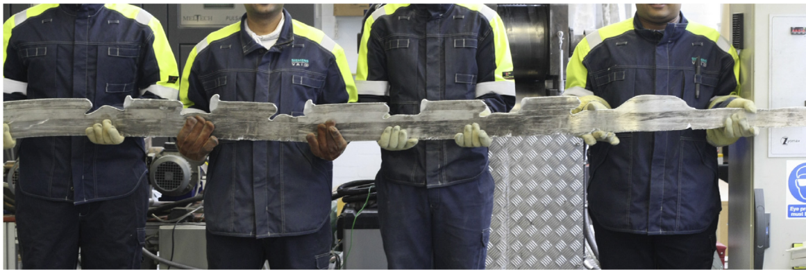
Fig. 8. Fastest width change in cast strip, showing immediate change in width from 130 to 75 mm and back.
