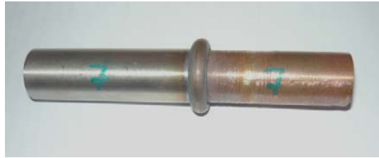
Fig.2. Friction welded joint (Sample 7)
