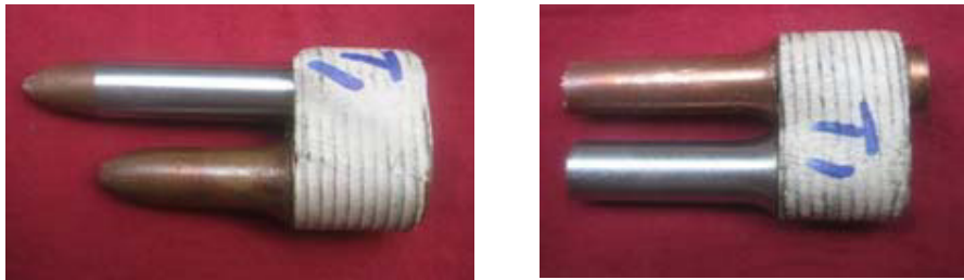
Fig.3. Macro photograph of tensile tested specimens of (a) ductile fracture in copper and (b) fracture in weld interface
