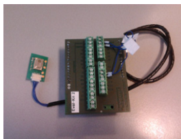
(a) Thermopile sensor used: Panasonic GridEye.
