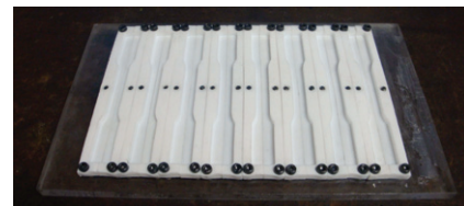
Fig.2 Mould for preparing epoxy specimens
