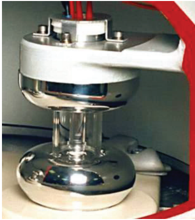
Fig. 1. Voltage sensor for 170 kV gas-insulated switchgear with a conventionally grown BGO crystal. [3].
