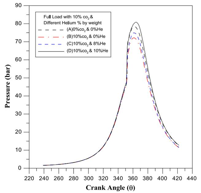
**Figure 7** Theoretical in-cylinder pressure of full load with 10% CO<sub>2</sub> and different % of Helium.
