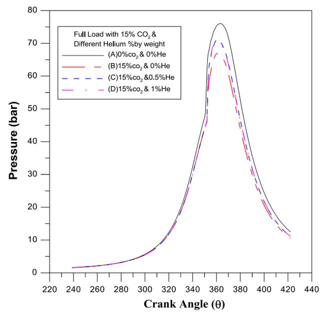
**Figure 8** Theoretical in-cylinder pressure of full load with 15% CO<sub>2</sub> and different % of Helium.
