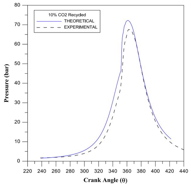
**Figure 4** The comparison in-cylinder pressure between theoretical and experimental of full load with 10% CO<sub>2</sub> recycled.
