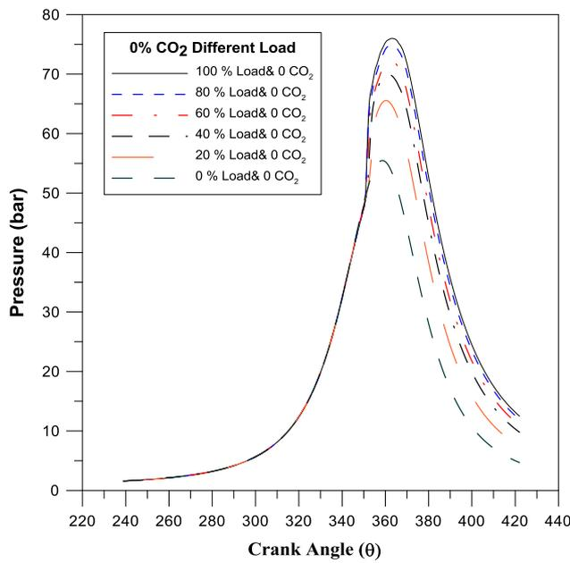
**Figure 5** Theoretical in-cylinder pressure of different load with 0.0% CO<sub>2</sub> recycled.
