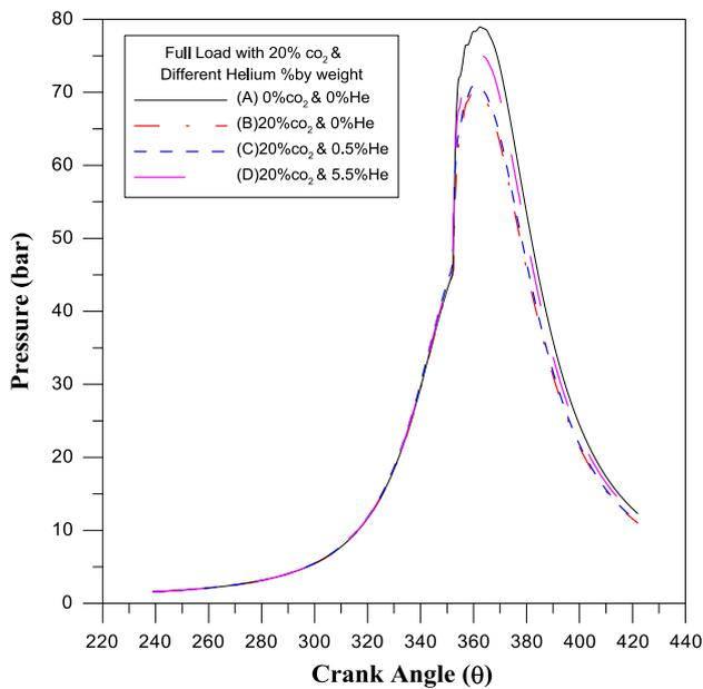
**Figure 9** Theoretical in-cylinder of full load with 20% CO<sub>2</sub> and different % of Helium.
