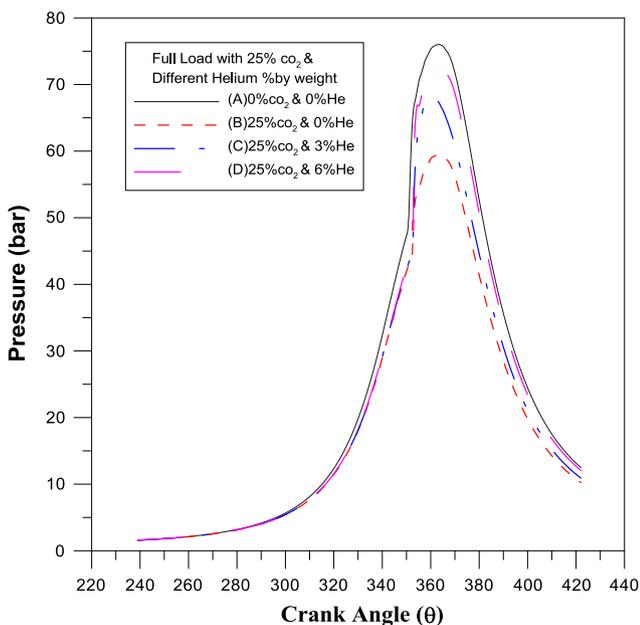
**Figure 10** Theoretical in-cylinder pressure of full load with 25% CO<sub>2</sub> and different % of Helium.
