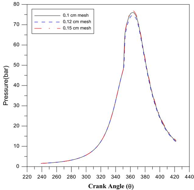
**Figure 3** The comparison in-cylinder pressure of different mesh.
