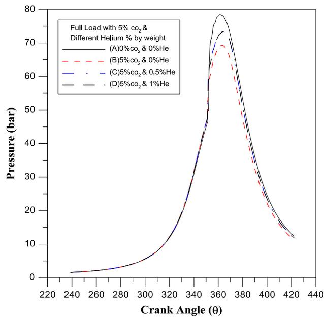
**Figure 6** Theoretical in-cylinder pressure of full load with 5% CO<sub>2</sub> and different % of Helium.
