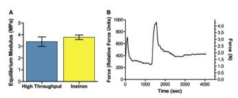
As the HTMS will be used for primary screening, slightly lower thresholds for accuracy are acceptable, as secondary screens follow on from 'hits' identified in primary screens. When the device was used to mechanically compress articular cartilage, the IFSR sensor captured the time-dependent stress-relaxation response (Fig 3B).
