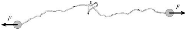
FIGURE 1 Diffusion of a tight knot along a stretched DNA molecule. The diagram illustrates the experimental design of the system (15). DNA is attached to the beads, which are manipulated by optical tweezers. The stretching force, F , is applied to the beads. The simulated conformation of a DNA molecule 3000 bp in length was used for the illustration. DNA molecules 16 times longer were used in the experiments.
