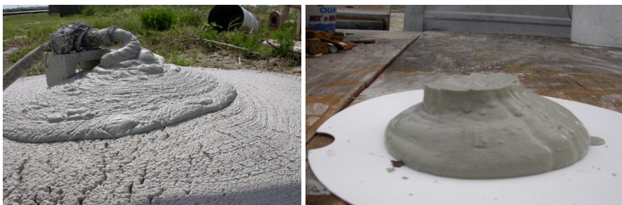
Figure 2. Sand/clay mix paste produced using deep cone thickener.
