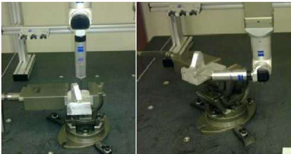
Fig. 5. CMM measurement of damaged part using touch-trigger probe
