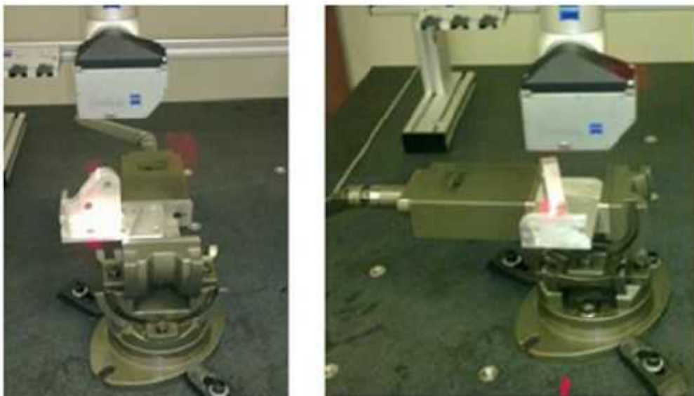
Fig. 6. Scanning of part at different degrees of freedom for fixture system
