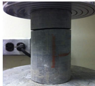
Fig. 7. Typical failure mode of specimens after direct tensile test.
