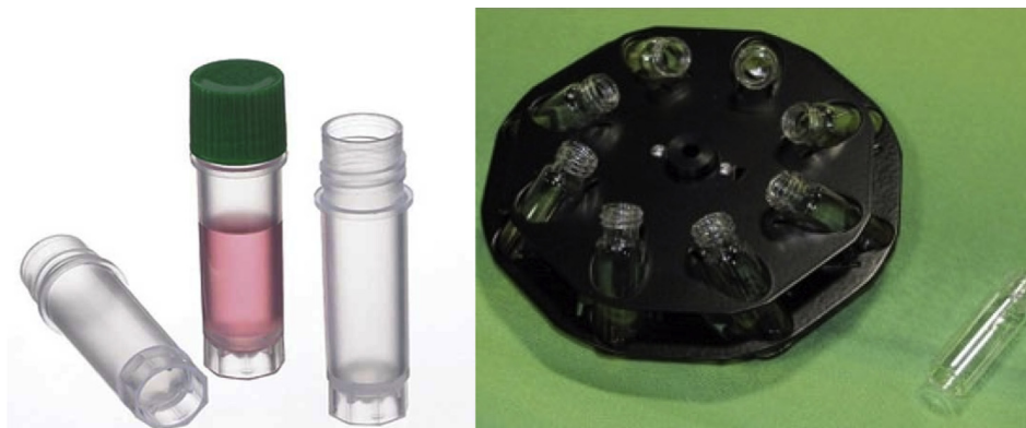
Figure 3. Shell vial that can be directly centrifuged.
