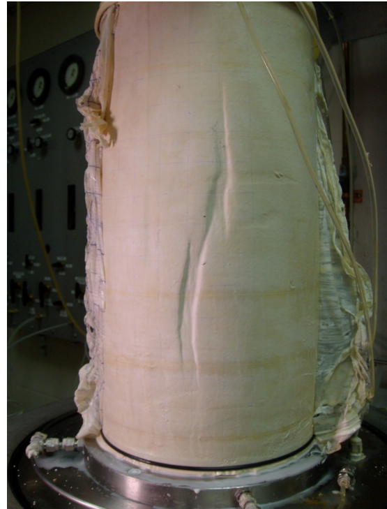
Fig. 16. Shear band pattern in hollow cylinder specimen with \alpha=0^\circ and b=0.79 . The outer layer of the membrane has been peeled off to clearly show the width and the sides of the “canyon” shear band oriented vertically in the direction of the major principal stress.
