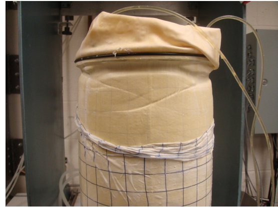
Fig. 20. Shear band pattern in hollow cylinder specimen with \alpha=90^\circ and b=1.0 . The outer layer of the membrane has been peeled off to clearly show the shear bands. A combination of “conventional” and “canyon” shear bands are observed.
