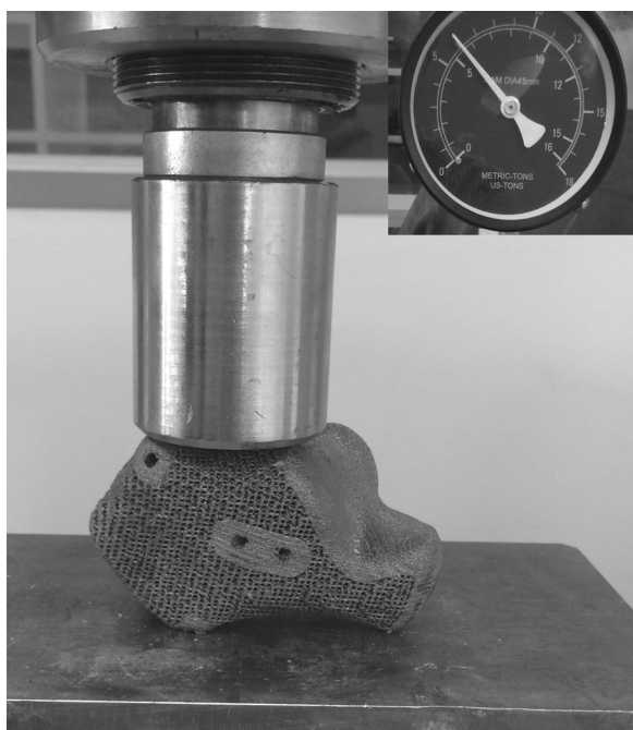
Fig. 2. A prototype of the calcaneal prosthesis showing an ability to sustain a load of over 6t.
