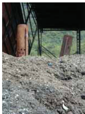
Fig. 25. Picture of tubes penetrated into the pile of industrial waste materials.
