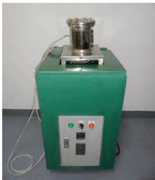
Fig. 1. Teflon-lined stainless steel autoclave unit.
