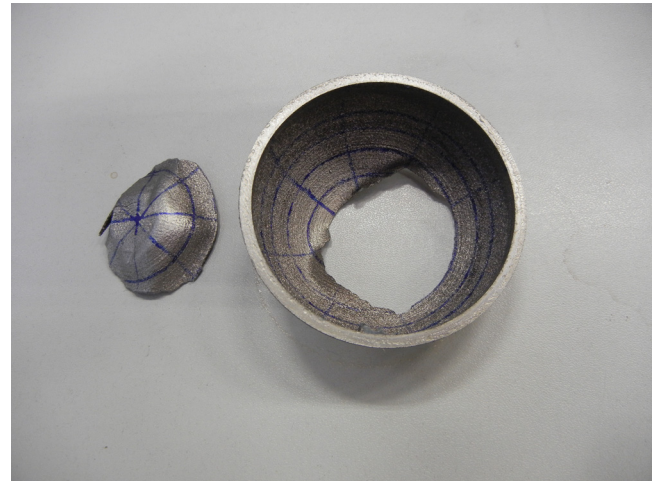
Fig. 12. Collapsed hemisphere of Batch 1.
