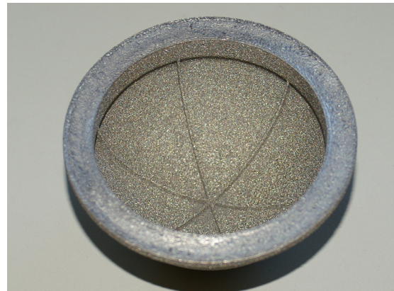
Fig. 6. Titanium hemisphere of Batch 2 with the joint surface not yet ground.
