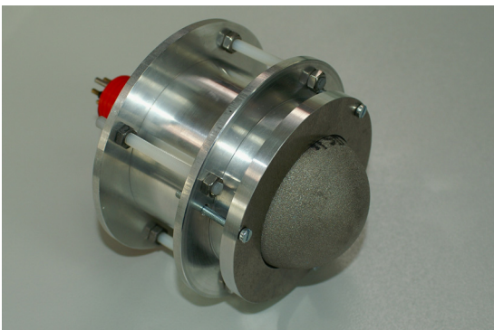
Fig. 4. The assembled pressure housing. The hemisphere, depicted in the right, joined to the camera housing.
