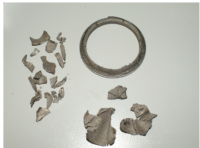
Fig. 13. Collapsed hemisphere of Batch 2.
