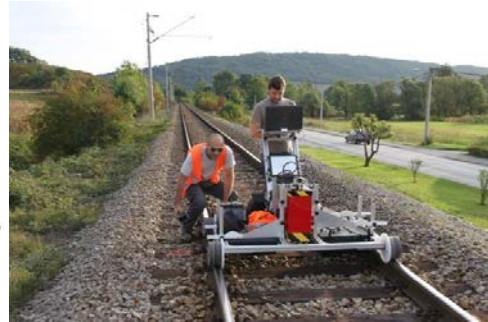
Fig. 6. Multichannel GPR system installed on the special vehicle.
