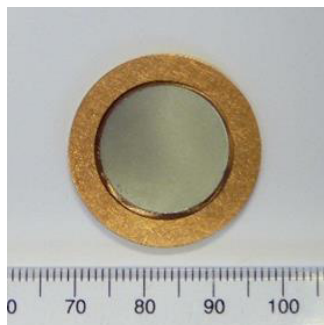
Figure 5 - Pressed-Sintered and Brazed Mo-Cu Target Disc for GE PETtrace Cyclotron.
