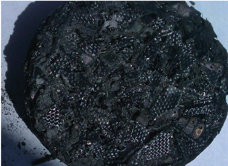
Figure 5. The co-pyrolysis solid residues of PCB in a tube furnace.
