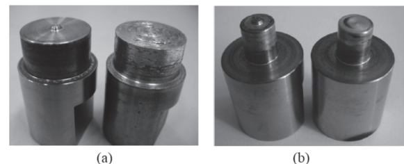
Fig. 2. “Pin” and “pinless” tool configurations: (a) d_s = 19 mm, (b) d_s = 8 mm
