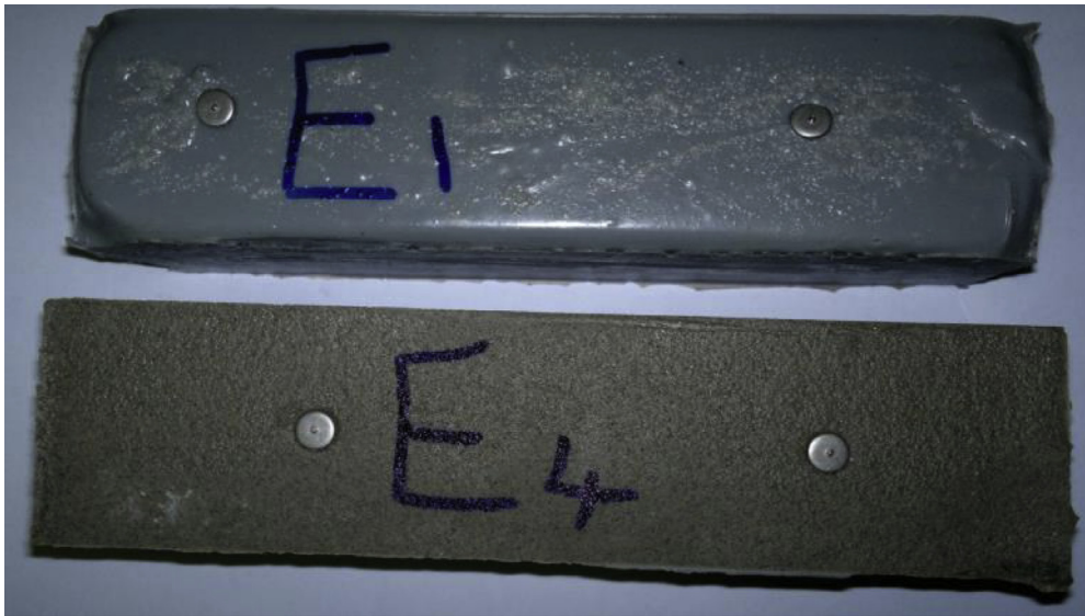
Figure 1. Consistency, instant inflating, and visible shrinkage of adhesive.
