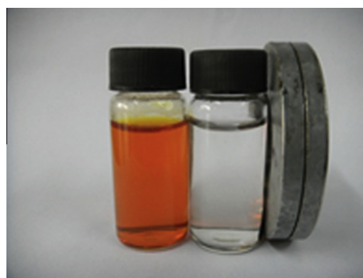
Figure 6b Photograph of CY solution (left), the solution after adsorption by GO-Fe 3 O 4 and separation with a magnet (right).
