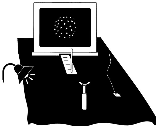
Fig. 1. Schematic view of the set-up. Subjects sat with their chin on a chin-rest, 80 cm from the monitor on which the stimulus was displayed. They changed the size and shape of the stimulus by moving the computer mouse. They indicated where they saw the stimulus by holding a tennis ball at that position (in complete darkness). The experimenter used a rod attached to a sliding ruler to measure the distance at which the subject held the tennis-ball. On some trials a table lamp provided a dim illumination of the surrounding. The table beneath the monitor and chin-rest was covered with a black cloth to minimise reflections.
