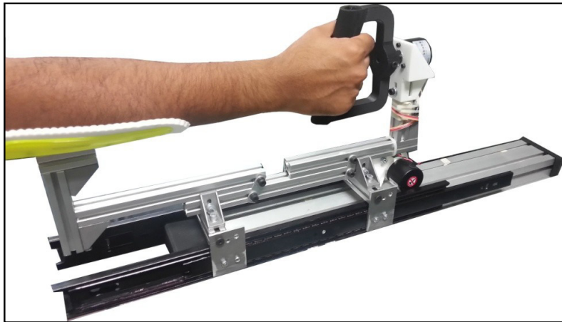
Fig. 1. Passive Upper Limb Assessment Device
