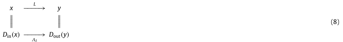
Fig. 1. The relationship between the logical states x and y and their representative physical states D_{in}(x) and D_{out}(y) , and the logical transformation L and the physical time evolution operator \Lambda_L .
