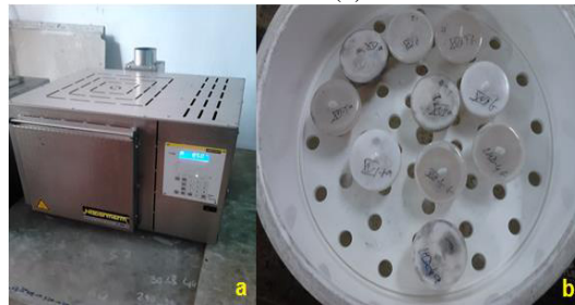
Fig. 5. (a) Muffle furnace to determine ash content of samples, (b) Sample kept in dessicator.
