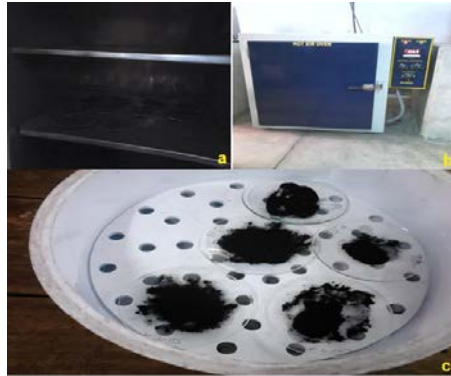
Fig. 3. (a) Samples in hot air oven, (b) Moisture Content Determination; (c) Samples kept in desiccator after taken out from oven.
