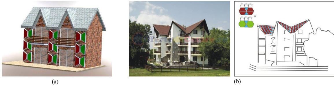
Fig. 5 Scaled representations of lego arrays integrated in residential buildings: (a) façade integration; (b) roof integration
