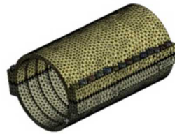
Fig.3. Bolt Pretension applied on bolts
