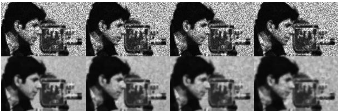
Fig.5 First row: a part of the “Cameraman” image with speckle noise with noise density level D = 0.02, 0.04, 0.06, 0.08 ; Second row: corresponding results of LBPD
