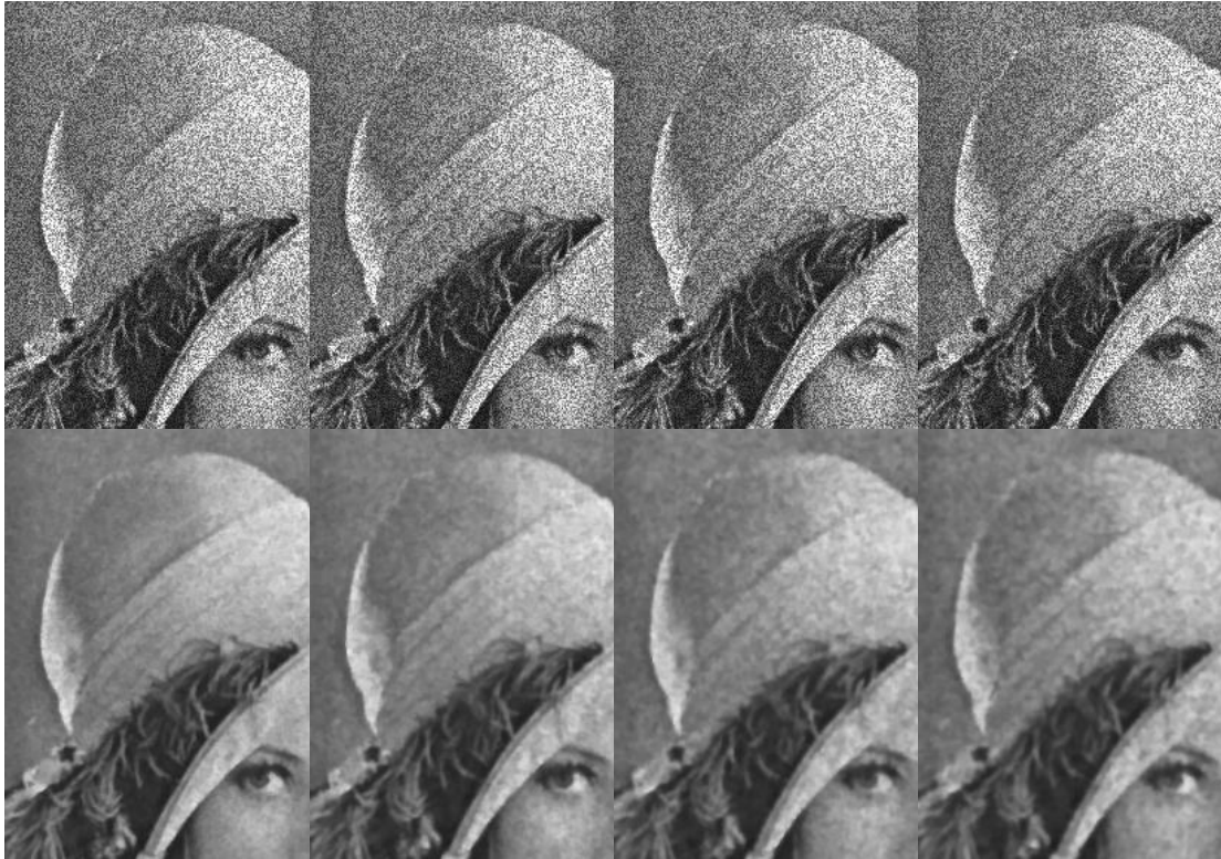
Fig.4 First row: a part of the “Lena” image with speckle noise with noise density level D = 0.02, 0.04, 0.06, 0.08 ; Second row: corresponding results of LBPD
