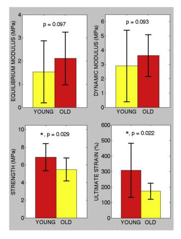
direction of collagen orientation. Specimens were kept hydrated and loaded under displacement control to 10% and 20% strain at 0.25%/sec and allowed to stress relax until equilibrium was reached, and finally loaded to failure. Equilibrium tensile modulus, dynamic tensile modulus, peak stress (strength) and strain at the point of peak stress were determined from the normalized load-displacement data. Wilcoxon rank sum tests were used to evaluate statistical significance of group differences.
