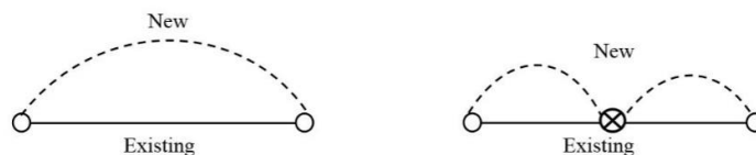
Fig.3. Addition of parallel pipe to existing pipe with no valve (left); and with valve (right).
