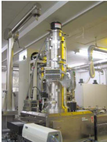
Fig. 3. Experimental column of multi-electron-beam system.
