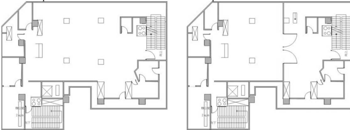
Fig. 2. non-compartment floor (left) can be improved by two sub-compartments with a fire rated metal rolling gate (right)
