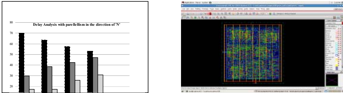
Fig. 4. (a) Chart showing the delays associated with delay types with different values of 'N'; (b) ASIC Floor plan
