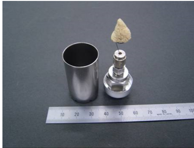
Fig. 4. Samples 2 and 3 shaped into 40-mg cones. This figure shows 40-mg samples on the combustion chamber platform.
