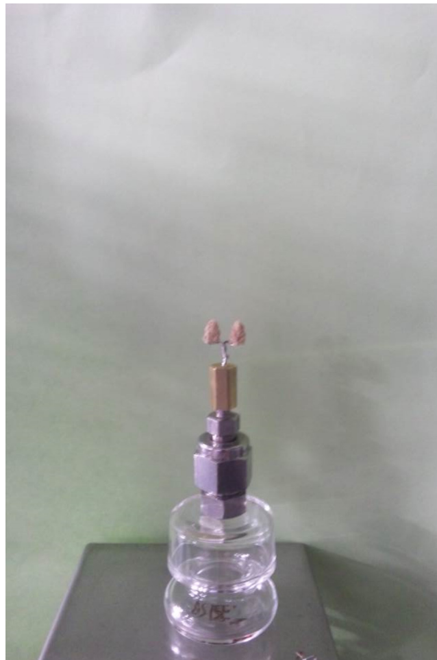
Fig. 3. Sample 1 moxa shaped into two 1-mg cones each placed side by side. This figure shows 1-mg samples on the combustion chamber platform.
