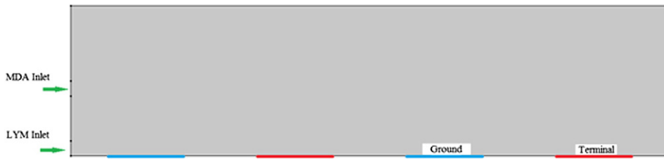
Fig. 4. Device with two different inlets for MDA case and LYM case.
