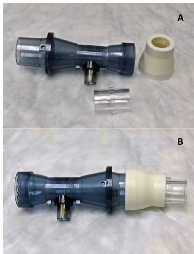
Fig. 2. Solving the connection conundrum. A) Mass flow sensor, flexible foam ventilator connector, and 15-15 mm tube connector; B) assembled connection.
