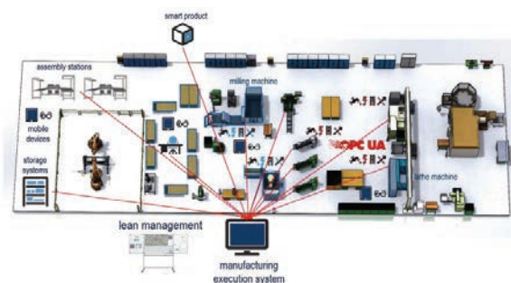
Figure 2: Infrastructure of the LPS learning factory
