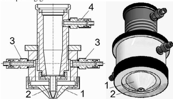
Fig. 2. Schematic view (a) and a 3-D view (b) of coaxial powder supply unit into the processing zone: 1,2 – replaceable nozzles; 3- powder and transportation gas inlets; 4- assist gas inlet.
