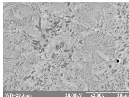
Fig. 9. Defects in the clad at optimal processing regimes ( $g=40^\circ$ ,  $mp=0.3g/s$ ,  $V=1.9mm/s$ ,  $DH=5mm$ )
