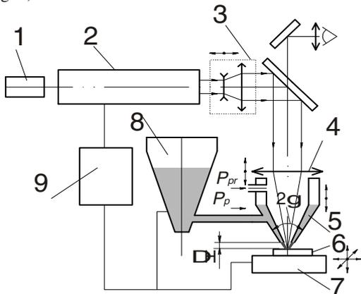
Fig. 1. Industrial laser equipment: 1- assist laser; 2- working laser 200 W; 3- telescope; 4- focusing objective; 5 -coaxial nozzle; 6 – workpiece; 7 – worktable with 3 coordinates; 8- powder feeder; 9 – control unit.
