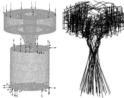
Fig.3. Mesh (a) and a particles trajectories (b) of coaxial powder supply system
