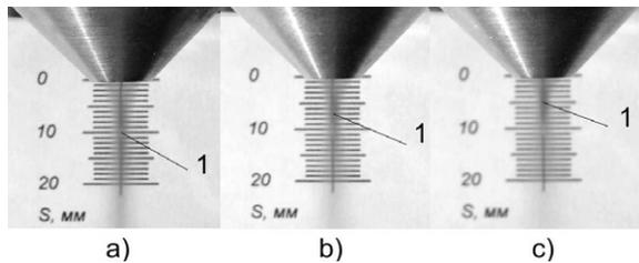
Fig. 5. General view of gas-powder streams after the nozzle exit, where a) - 30° nozzle forming angle; b) 40° nozzle forming angle; c) - 50° nozzle forming angle; 1- minimal cross-section of gas-powder stream.
