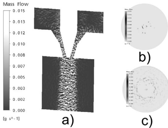
Fig. 4. Distribution of the concentration of powder mixture along the axis of distribution (a) and in cross-section (b, c) at the nozzle exit (b) and in powder focusing spot (c).
