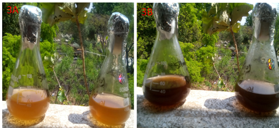
Figure 3 Each flask containing individual fungal filtrate and \text{AgNO}_3 , (3A) fungal filtrate with 100 Mm \text{AgNO}_3 10 min after exposed to sunlight (3B) fungal filtrate with 100 Mm \text{AgNO}_3 20 min after exposed to sunlight.
