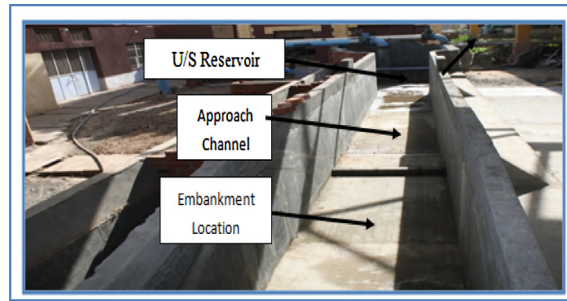
(a): The Upstream of the Flume
