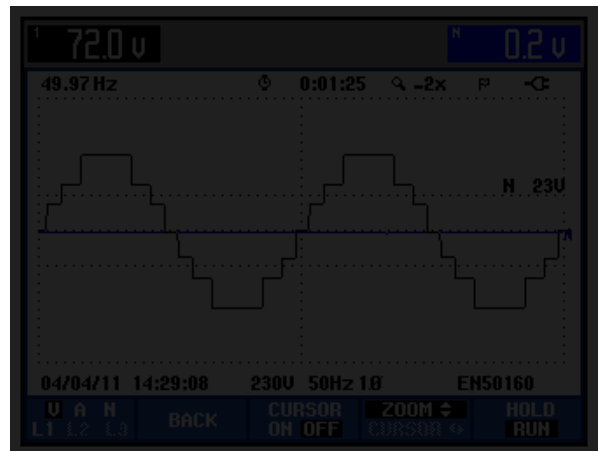
Fig. 13: Harmonic content output voltage waveform \theta_1=9.06^\circ , \theta_2=28.52^\circ , and \theta_3=55.05^\circ
