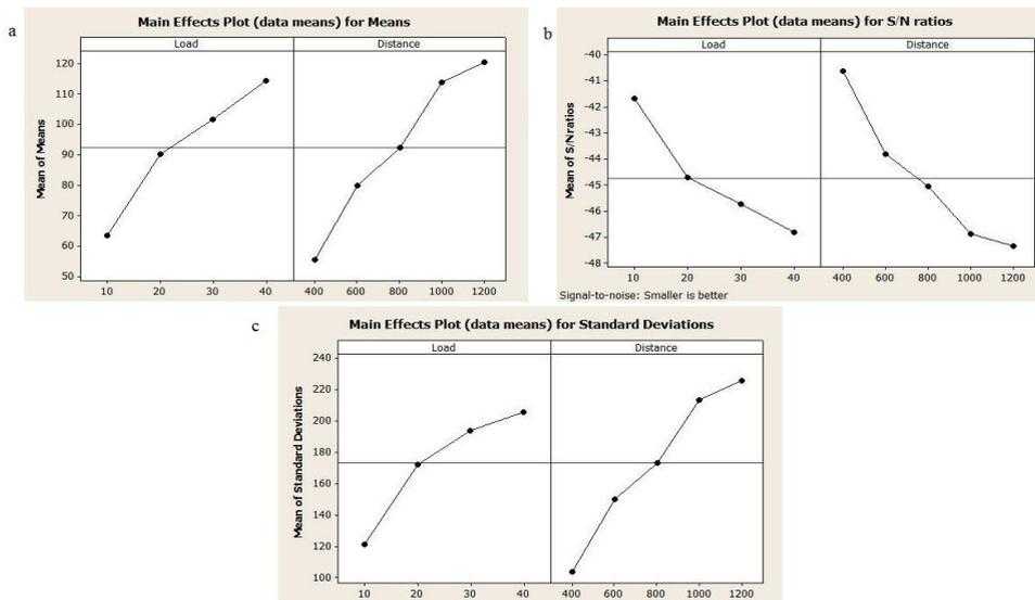
Fig. 4. Analysis of Wear behaviour of AA7075/ Al<sub>2</sub>O<sub>3</sub> Compositions using Taguchi method.
