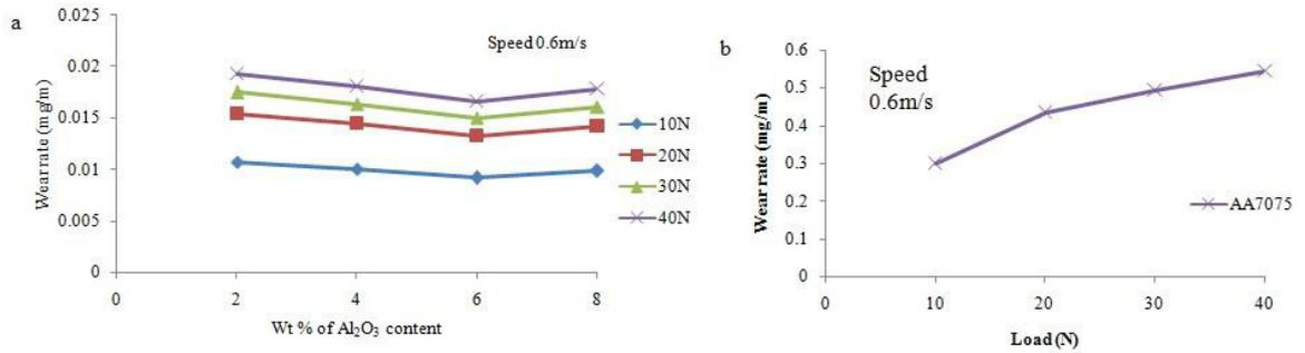
Fig. 2. Variation of Wear rate under various load Conditions (a) AA7075/ Al<sub>2</sub>O<sub>3</sub> (b) AA7075 composites.
