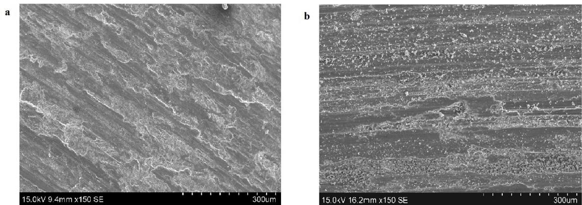
Fig. 3. Worn surface morphology of (a) AA 7075 (b) AA 7075 / 6 Wt % of Al<sub>2</sub>O<sub>3</sub> composites at 0.6 m/s and 1200 meters sliding distance.
