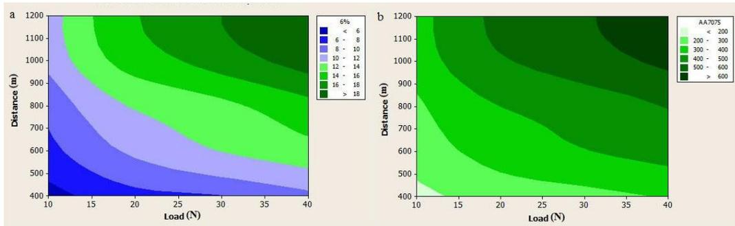
Fig. 5. Contour plot of variation in wear mass loss (a) 6 Wt % of  $\text{Al}_2\text{O}_3$  (b) AA7075 composites.
