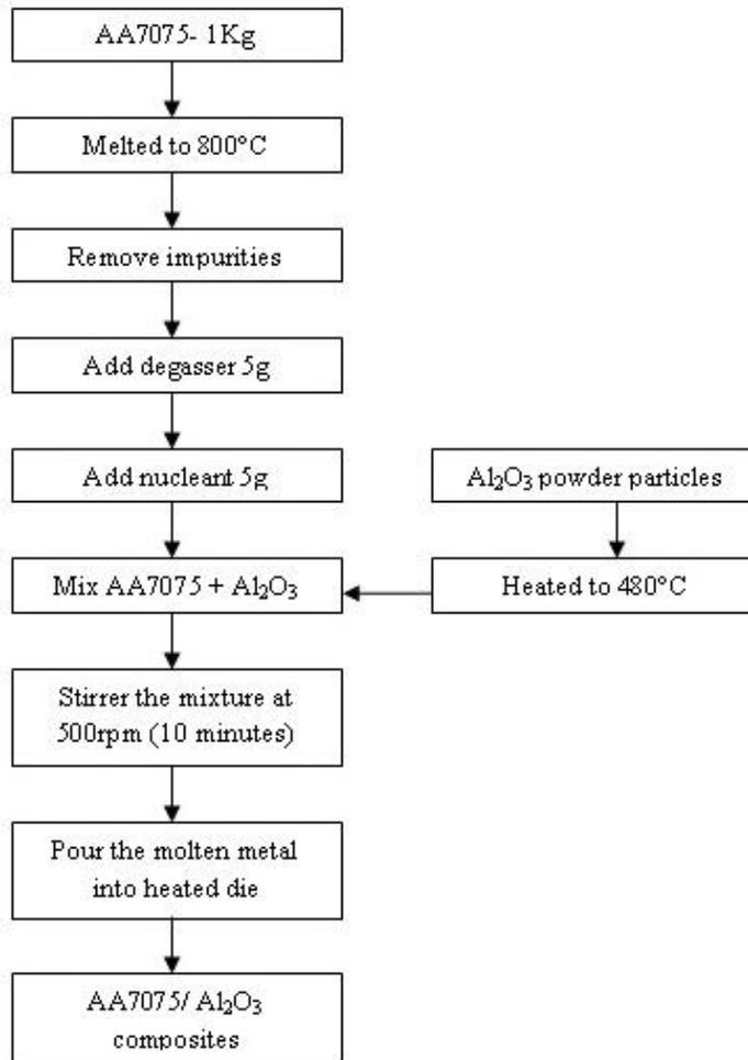
Fig. 1. Steps involved in stir casting process.
