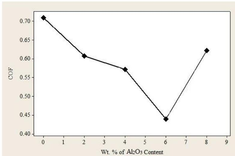
Fig. 6. Variation of COF with increasing Wt % of  $\text{Al}_2\text{O}_3$ .
