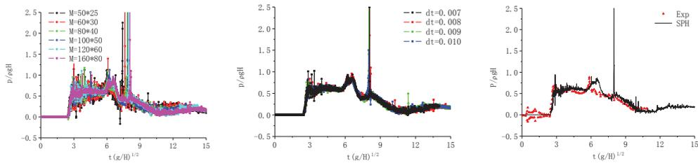
Fig. 3. Pressure time history comparisons of different particle numbers (left), different stepping length (middle), experimental results(right).
