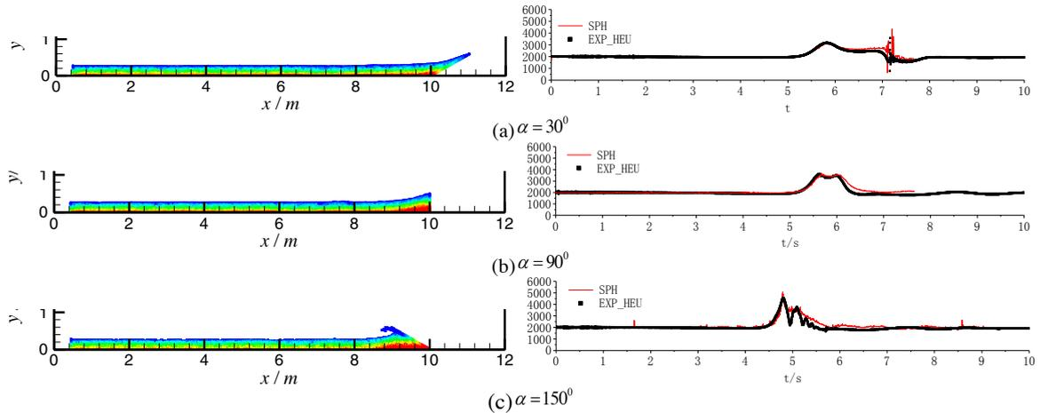
Fig.5 Pressure distribution of different slope angles and wave impact pressure comparison
