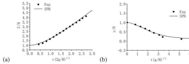
Fig. 1. Water wave front comparison (a); water wave height comparison (b).
