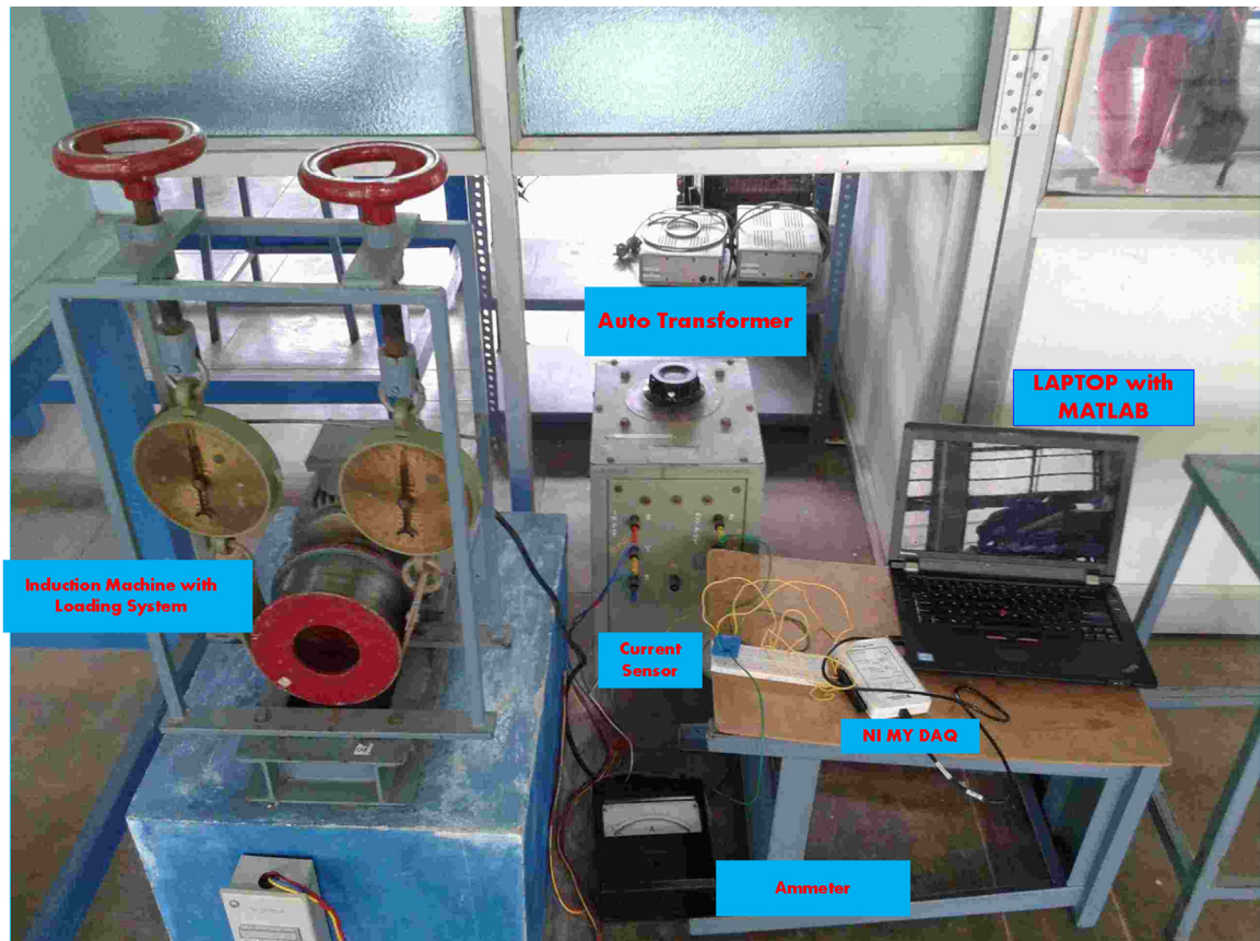
Fig. 6. Experimental setup for bearing fault detection.
