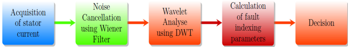
Fig. 3. Block diagram of proposed bearing fault detection topology.
