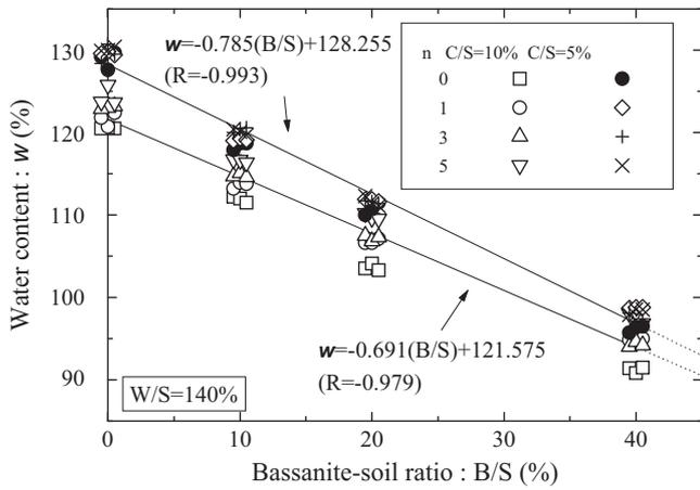
Fig. 8. Influence of Bassanite–soil ratios (B/S) for each cement–soil ratio (C/S) used on water content of stabilized soil specimens subjected to wetting and drying cycles ( $n$ ).
