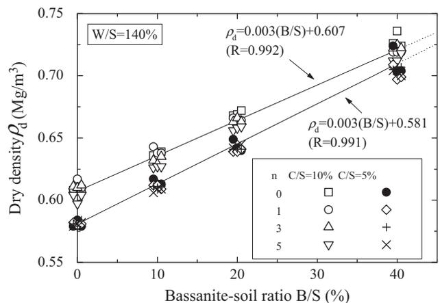
Fig. 7. Influence of Bassanite–soil ratios (B/S) for each cement–soil ratio (C/S) used on dry unit weight of stabilized soil specimens subjected to wetting and drying cycles ( $n$ ).
