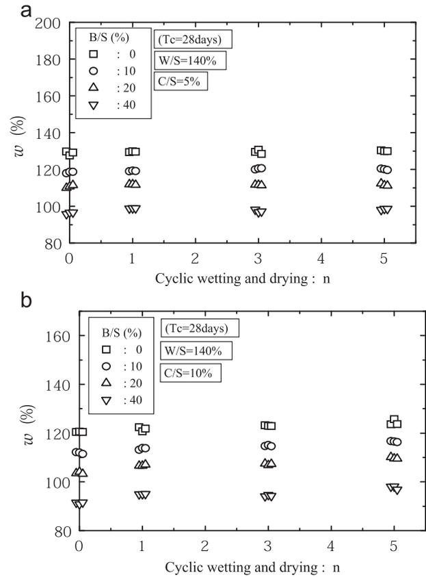
Fig. 10. Influence of wetting–drying cycles ( $n$ ) on water content of soil specimens stabilized with different Bassanite–soil ratios (B/S) for each cement–soil ratio (C/S) used. (a) In case of cement–soil ratio (C/S) of 5%. (b) In case of cement–soil ratio (C/S) of 10%.
