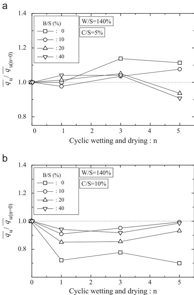
Fig. 6. Influence of number of wetting–drying cycles ( $n$ ) on durability index for soil samples stabilized with different Bassanite–soil ratios (B/S) for each cement–soil ratio (C/S) used. (a) In case of cement–soil ratio (C/S) of 5%. (b) In case of cement–soil ratio (C/S) of 10%.
