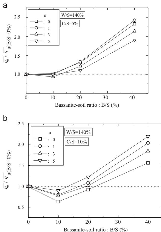
Fig. 5. Effect of Bassanite–soil ratios (B/S) for each cement–soil ratio used on durability index for stabilized soil samples subjected to wetting–drying cycles. (a) In case of cement–soil ratio (C/S) of 5%. (b) In case of cement–soil ratio (C/S) of 10%.
