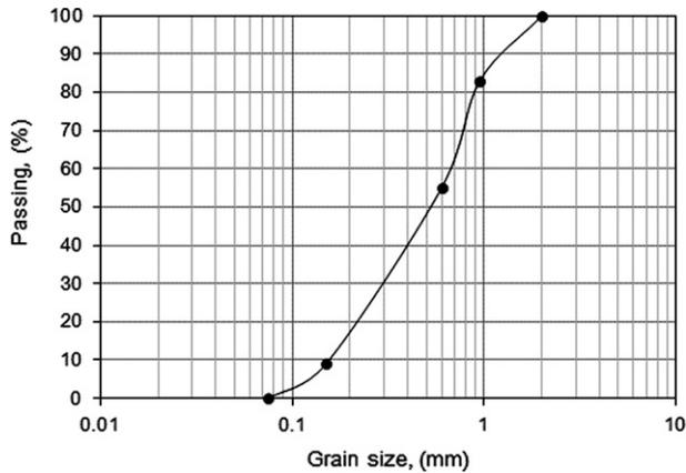
Fig. 1. Grain size distribution curve for Bassanite.
