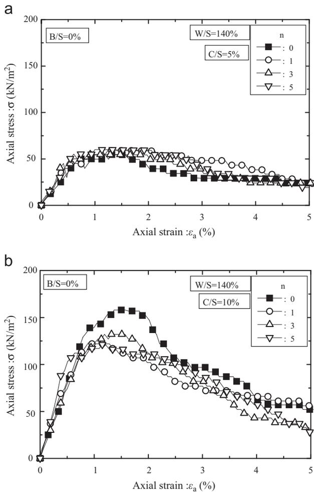
Fig. 2. Stress–strain relationships for samples stabilized with only furnace cement and subjected to wetting–drying cycles ( $n$ ). (a) In case of cement–soil ratio ( $S/C$ ) of  $5\%$  and without Bassanite ( $B/S=0$ ). (b) In case of cement–soil ratio ( $S/C$ ) of  $10\%$  and without Bassanite ( $B/S=0$ ).
