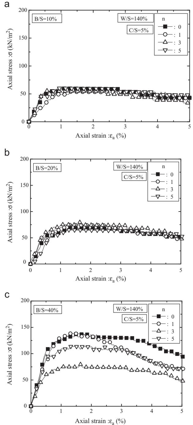
Fig. 3. Stress–strain relationships for soil samples stabilized with different Bassanite–soil ratios ( $B/S$ ) at cement–soil ratio ( $C/S$ ) of  $5\%$  and subjected to wetting–drying cycles ( $n$ ). (a) In case of Bassanite–soil ratio ( $B/S$ ) of  $10\%$ . (b) In case of Bassanite–soil ratio ( $B/S$ ) of  $20\%$ . (c) In case of Bassanite–soil ratio ( $B/S$ ) of  $40\%$ .
