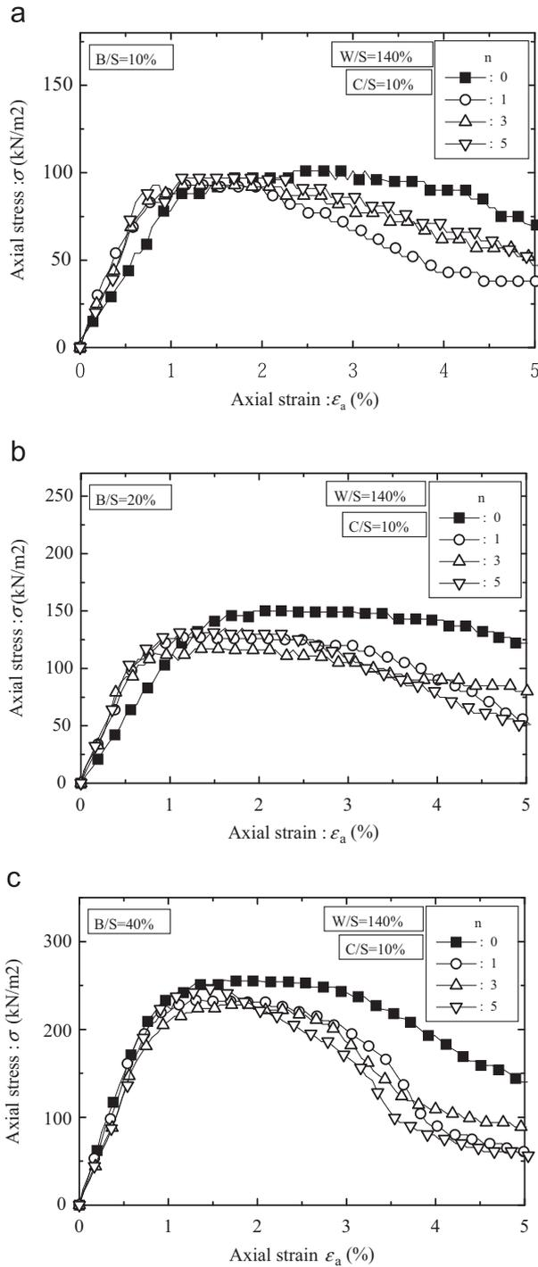
Fig. 4. Stress–strain relationships for soil samples stabilized with different Bassanite–soil ratios (B/S) at cement–soil ratio (C/S) of 10% and subjected to wetting–drying cycles ( $n$ ). (a) In case of Bassanite–soil ratio (B/S) of 10%. (b) In case of Bassanite–soil ratio (B/S) of 20%. (c) In case of Bassanite–soil ratio (B/S) of 40%.
