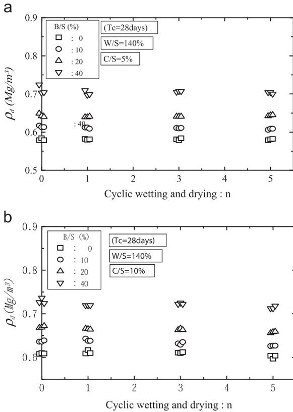
Fig. 9. Influence of wetting–drying cycles ( $n$ ) on dry unit weight of soil specimens stabilized with different Bassanite–soil ratios (B/S) for each cement–soil ratio (C/S) used. (a) In case of cement–soil ratio (C/S) of 5%. (b) In case of cement–soil ratio (C/S) of 10%.
